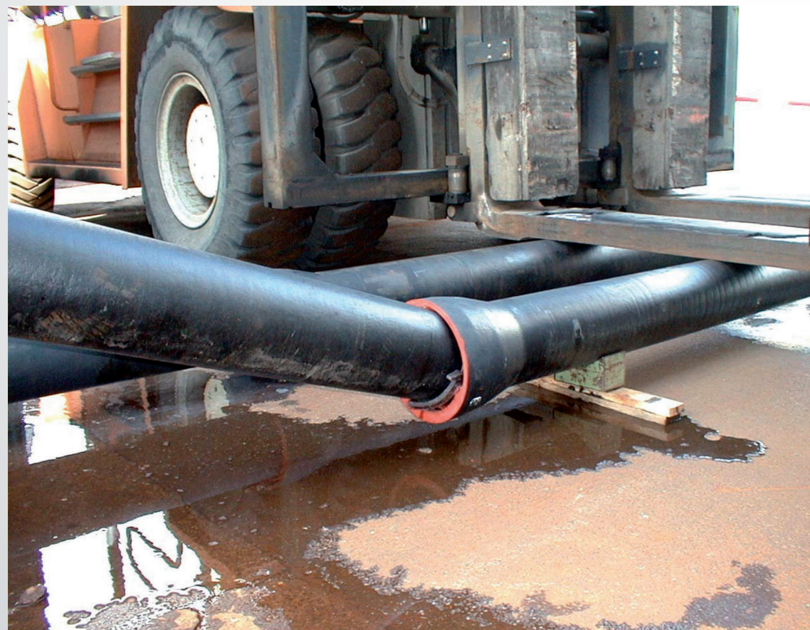
Deflection test: save connection up to 24°
