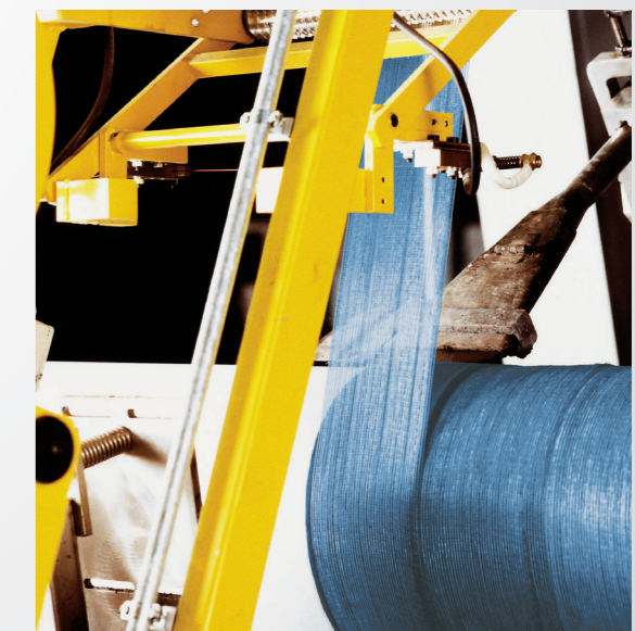
Application of the ZMU coating in the factory
